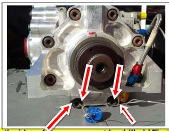
Both sides of the screw must be drilled / First seal max 20mm
