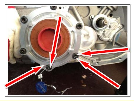
Both sides of the screw must be drilled / First seal max 20mm
